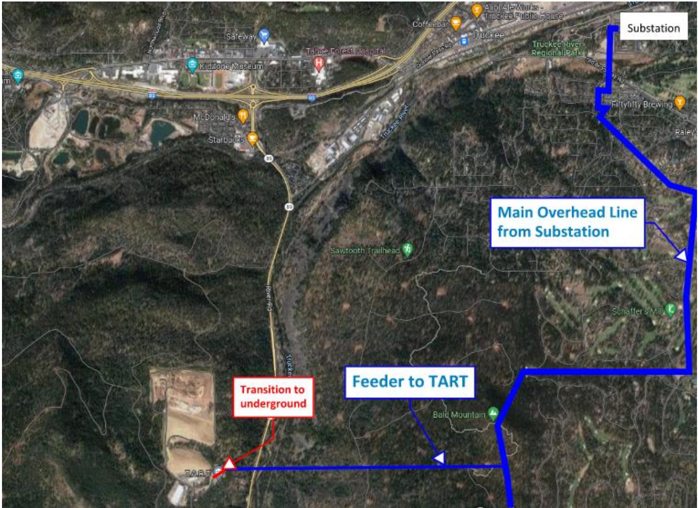
Figure 4-4. Feeder from Substation to TART
